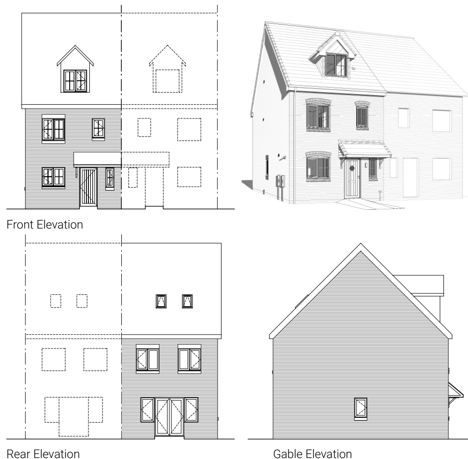
Figure 3. House type “Room-in-roof semi-detached”; dual aspect; the South elevation, at the rear, is the most highly glazed façade. This house type can be assessed using the Simplified Method in moderate risk locations: it passes once more window panes are made openable - see details in Worked Example, section 8.
